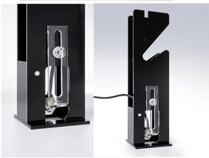
once the sensor is on the mounting bracket, you can install it on to the upper part(1) of the roller frame with supplied nylon screw
