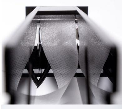
The Loose end of the fleece should be guided through the roller frame (2) as shown
