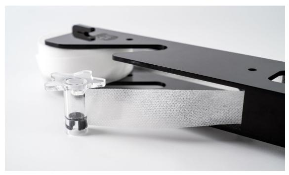
Guided the loose end of the fleece through the roller frame and secure the fleece onto the twist-lock tube.
